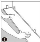
2. **First row, second plank:** Place the plank gently and close to the short side of the previous plank. Fold down the plank starting from the opposite
